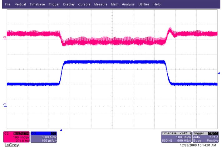
**Transient Response  $V_{IN}=12V, I_o=3A$  Step from 1.5A~3A~1.5A( $V_{o2}$ )**
