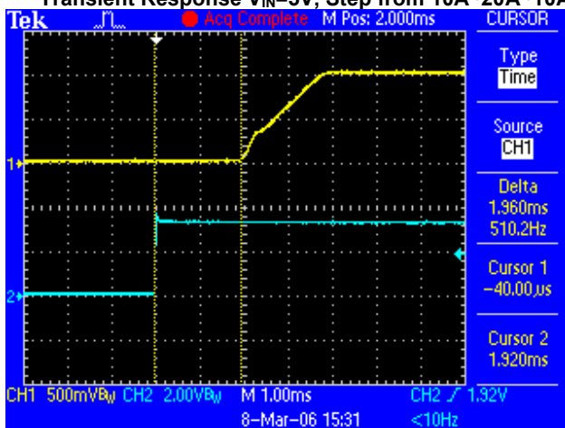
Start-up V_{IN}=3.3V , I_O=15.6A (resistive load)
